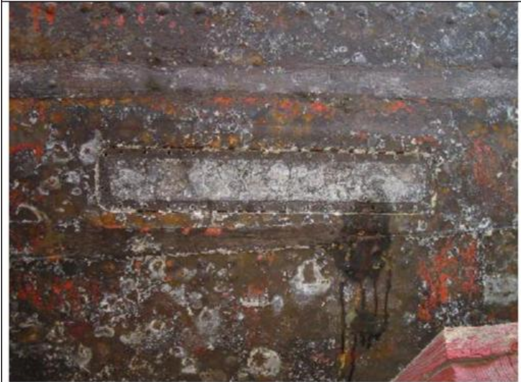
The port or starboard side hull openings for the SQS501 transducer look like this. This photo of HAIDA's hull was taken when she was in drydock in 2003. The hull has just been power washed, hence the lack of paint. ( Photo by Jim Brewer )
