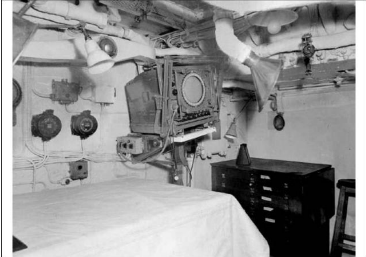
Operations Room Aboard HAIDA in 1946: Forward bulkhead showing the 293M PPI slave display. Through a large magnifying glass fitted in the deckhead of the Operations Room starboard side, bridge personnel could read the plot table and the PPI display. The front of the PPI display is shown with the mirror mounting frames folded back and in the stowed position. When in use, the frame was extended and a mirror would be inserted into the frame and positioned so the screen could be viewed from above. The Plot Table is shown with the dust cover in place. (RCN photo #1749-56)
