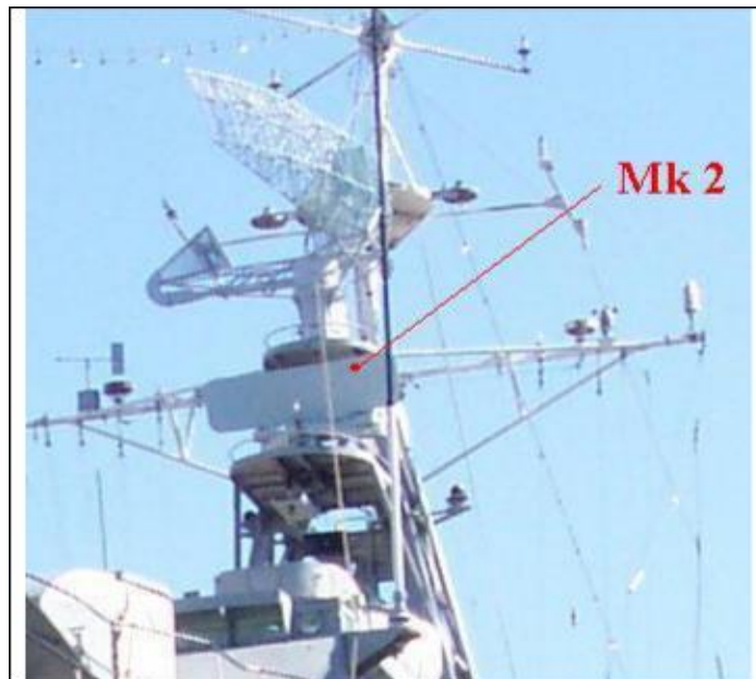
Location of the Sperry MK II scanner (antenna) on the foremast. (Photo by Jerry Sullivan)
