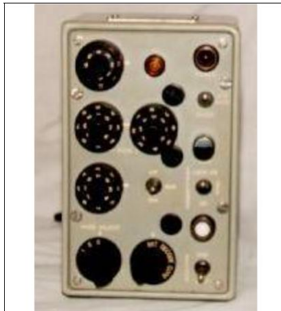
UPA-24/C1008 Control. This was the control box for the group video decoder. Located in the Ops Room, it controlled the mode of transmission (ie mode 1, 2 or 3) and the 'squawk' code assigned to each particular ship. (Photo by Jerry Proc)
