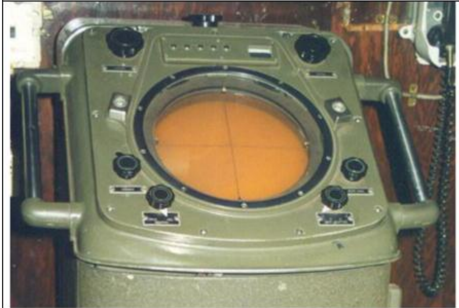
This is the Sperry MkII PPI display as fitted in the Ops Room of HMCS HAIDA. (Photo by Jerry Proc)
