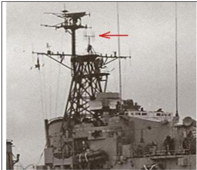
Aerial Outfit ASS on HAIDA during her first tour of duty in Korea. (Photo courtesy RCN)
