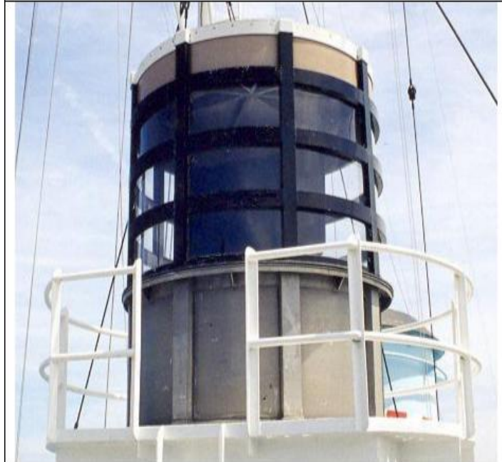
Perspex enclosure for the 271 radar antenna. This is a recreated enclosure found on HMCS Sackville. (Photo by Jerry Proc)
