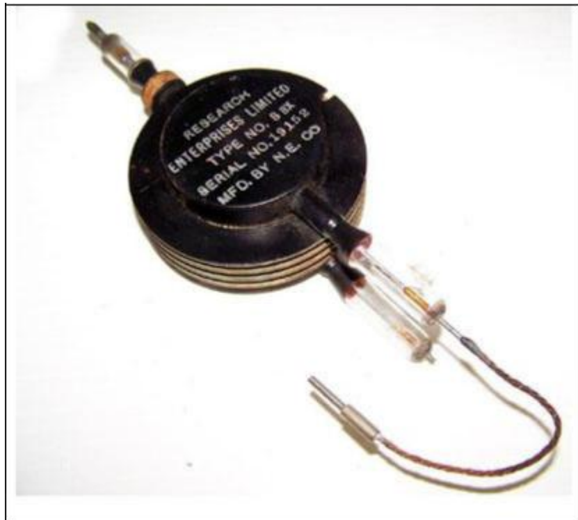
This is the same type of 10 cm magnetron brought to North America by the Tizard Mission in 1940. This specific example is Canadian Type 8 BX s/n 19152. It was manufactured by Northern Electric for Research Enterprises Ltd, a Canadian Crown Corporation. One of the filament leads is missing. (Photo by Jacques Hamel, VE2DJQ, Le Musée Québécois de la Radio)
